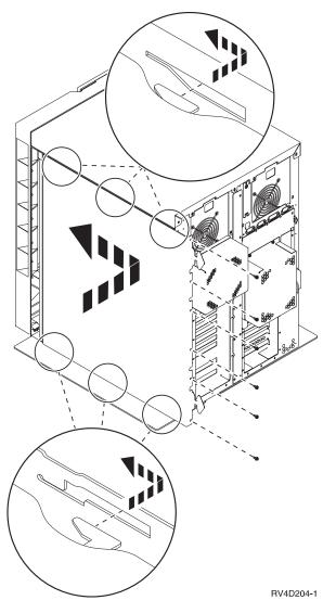
Figure 7. Install Side Cover
